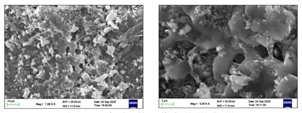
Figure 5. SEM of catalyst with magnification (a) 1000× (b) 5000×
